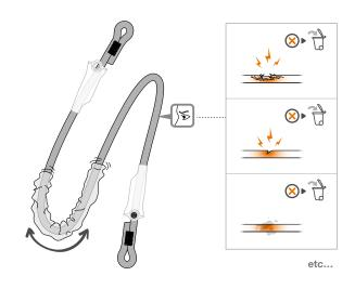
• Do a tactile inspection of the core along the full length of the rope (hard spots, swelling, soft or crushed areas...).
