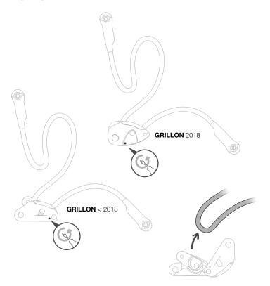
• Look for wear and damage on the sheath due to use (cuts, fuzziness, signs of chemicals...). Move the protective sleeve to see the rope's condition along its entire length.
