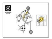
The AUTO-LOCK system automatically locks the rope when the handle is not in use.
