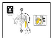
The AUTO-LOCK system allows users to easily position themselves at a workstation without having to manipulate the handle or tie off the device: as soon as the user releases the handle, the rope is automatically locked in the device.
