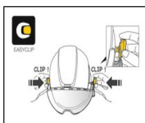
Installation is quick and easy, thanks to the included EASYCLIP attachment system.
