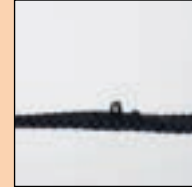
Loop pulled on smooth webbing
