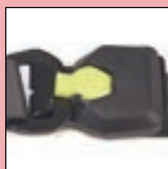
Triple Lock buckle with broken button
