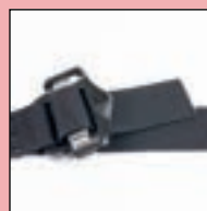
Webbing termination missing
