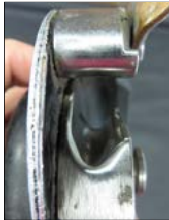
• Cam groove worn to wear indicator
