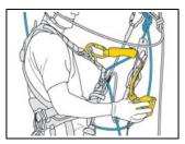
The connection arm makes the system drop-resistant when passing intermediate anchors.
